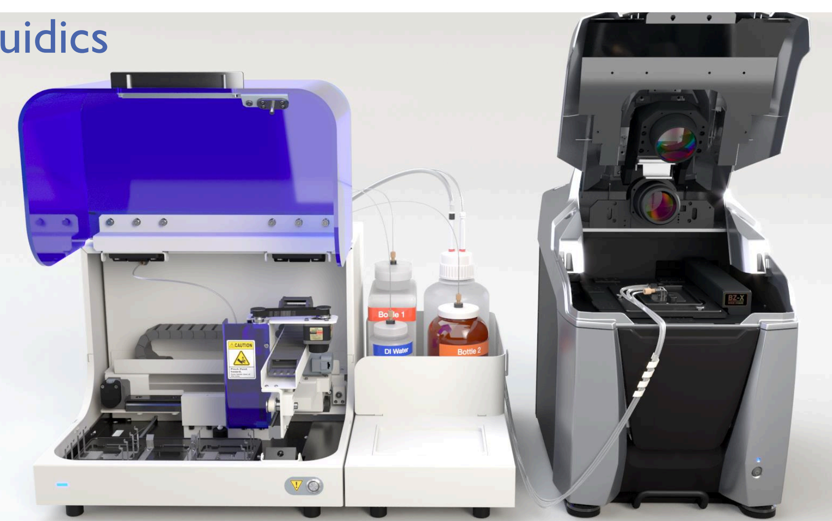
Figure 3: The iterative process is automated through Akoya's microfluidics platform (left) that can be integrated with a widefield epifluorescence microscope as shown above (right).
